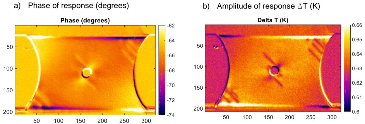
Figure 2: TSA Results tension/shear load case 10 Hz loading frequency
