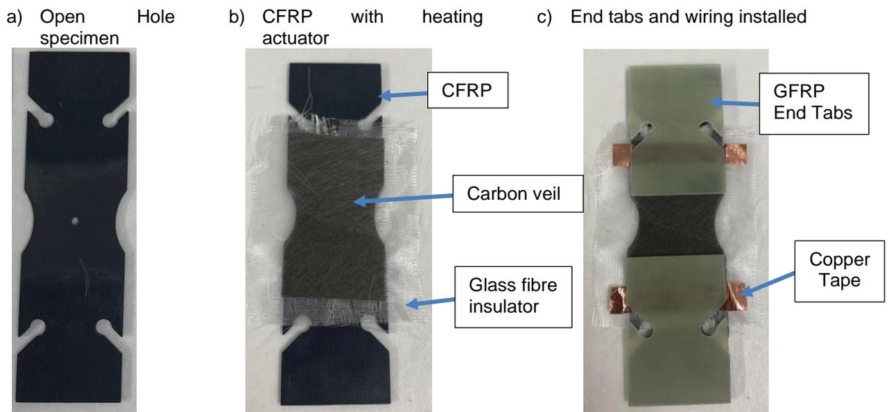
Figure 1: Specimen Configuration
