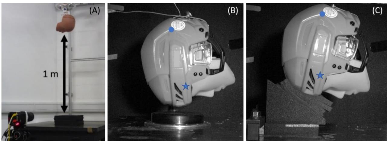
Fig. 1: (A) Free-fall drop test setup, (B) Front site, flat MEP pad surface just before impact (C) Front site, oblique 72 mm foam during impact with FrontBoss (★) and RearBoss (●) impact sites marked.
