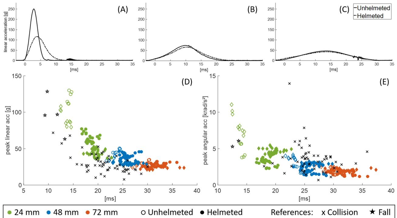
Fig. 2: Linear acceleration vs. time curves for flat surface, unhelmeted and helmeted Front site impacts onto the (A) MEP pad, (B) 48 mm foam layer, and (C) 96 mm foam layer; Peak linear (D) and angular (E) accelerations vs. impact duration for all impact scenarios onto the 45° oblique surface; filled markers represent helmeted impacts and unfilled markers represent unhelmeted impacts, black markers represent reference values of concussive impacts recreated in a laboratory environment [7].
