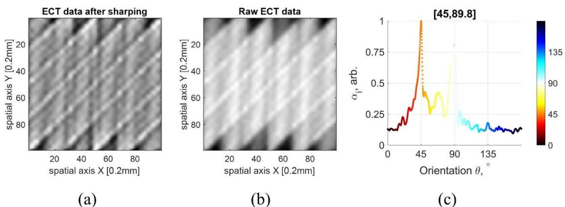
Figure 1 Primary results:(a) 2D sharpening gaussian filtering on FEM data, (b) FEM data exported from COMSOL,(c) radon transform for orientation inversion(peaks are at 45 and 89.8 [degs])
