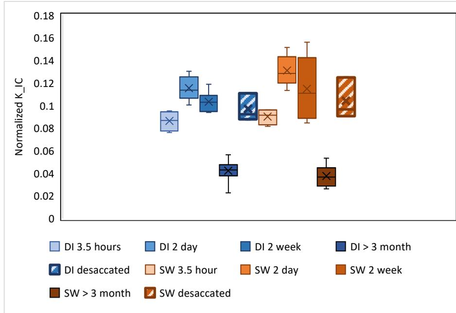
Fig.1 Dynamic fracture values normalized by ambient results, DI = distilled water and SW = sea water.
