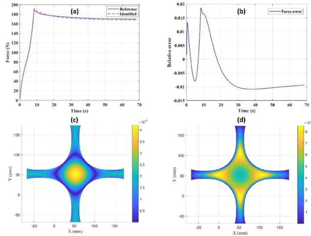
Figure 2: comparison of the obtained results with the reference data: (a) global force, (b) relative error of the global force, (c) relative error of the first in-plane principle stretch and (d) relative error of the second in-plane principle stretch
