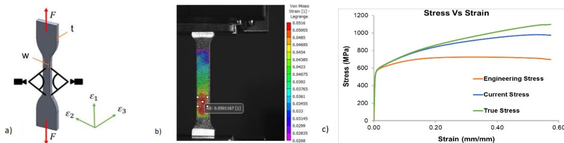
Figure 1: a) System set up for uniaxial tests, b) Data extraction using DIC approach, c) stress-strain curves of stainless steel 316L under quasi-static load.
