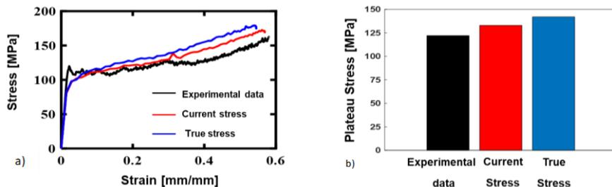
Figure 2: a) Stress - strain curves for the three different scenarios and b) plateau stress.
