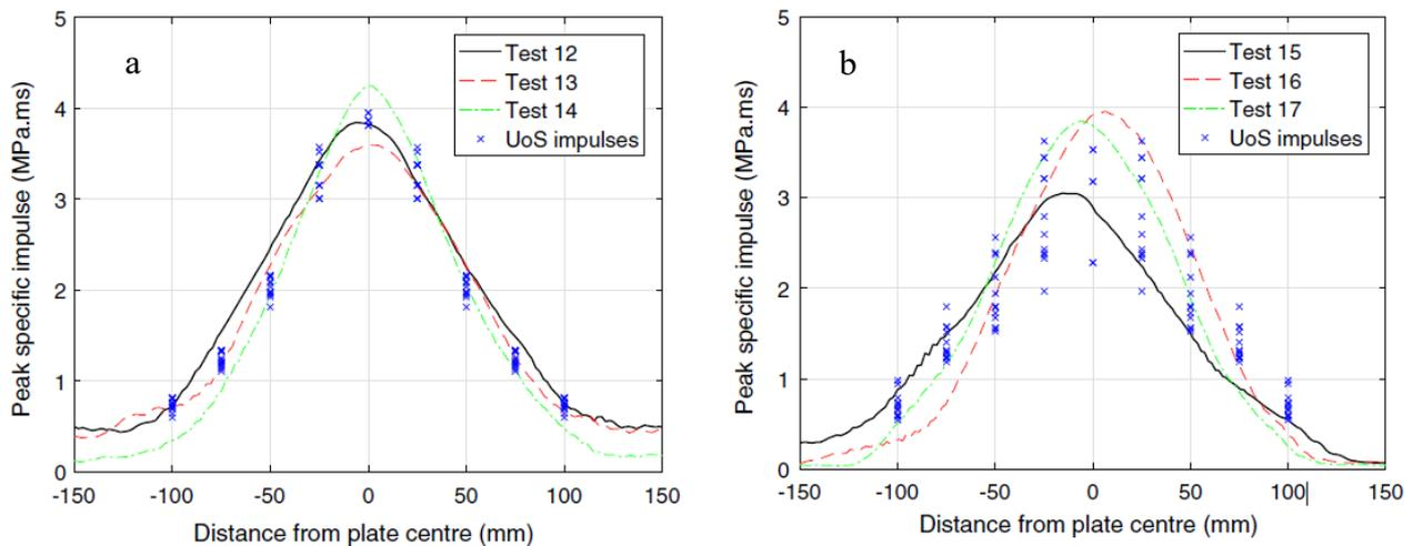
Figure 2: Measured (COBL) and inferred (BISRU) specific impulse distributions for (a) spherical detonations (b) cylindrical detonations
