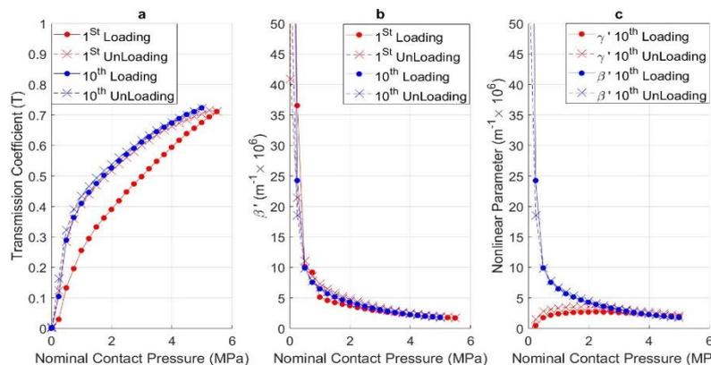
Figure 2. Reflected and transmitted signal from/through a dry rough contact as nominal pressure increases for the 1<sup>st</sup> and 10<sup>th</sup> loading/unloading cycles: (a) transmission coefficient; (b) transmitted nonlinear parameter  $\beta'$ ; (c) reflected and transmitted nonlinear parameters at the 10<sup>th</sup> loading/unloading cycle.
