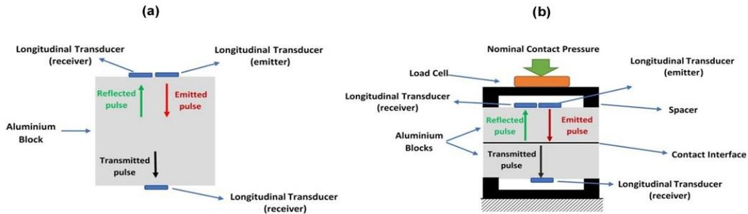
Figure 1. Schematic diagram of the apparatus: (a) continuum aluminium block; (b) dry rough contact.
