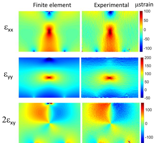
Figure 2: Comparison between finite element and experimental surface strains.
