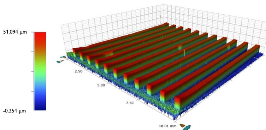
Fig. 1: Optical profilometer scan of structured polycarbonate sample produced by injection moulding, nominal sample area 10x10 mm.
