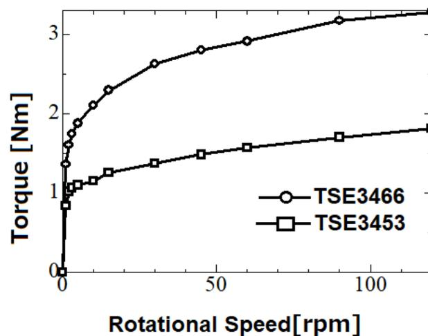
Fig.2 Torque vs. rotational speed curve using TSE3466 and TSE3453 silicon rubber elastomers
