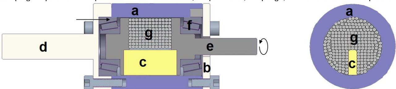
Fig. 1 Schematic diagram of rotary damper a. Body, b. Cover, c. Rotor, d. Holder, e. Shaft, f. Bearings, g. elastomer particles
