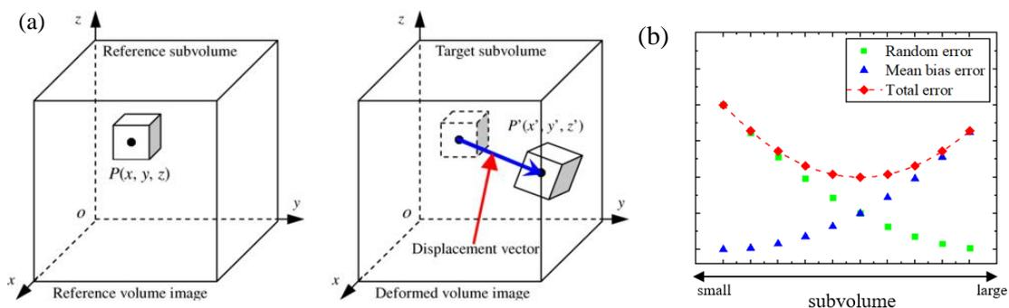
Figure. 1. SA-DVC: (a) schematic figure of DVC, (b) schematic figure of V-shaped total error
