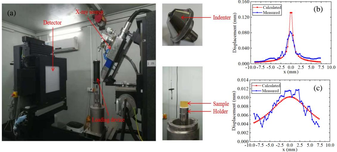
Figure 2. Experiment results: (a) experiment setup, (b) comparison at 0.3 mm load,  $z = 5.5$  voxel, (c) comparison at 0.3 mm load,  $z = 195.5$  voxel
