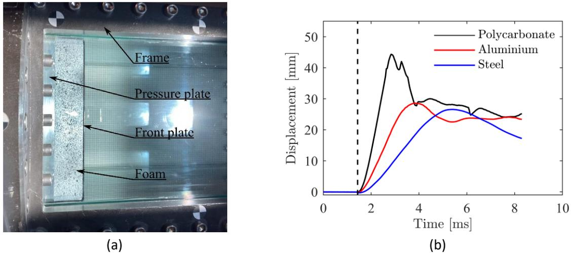
Figure 2. (a) Details of the experimental set-up with EPP-backed plates, and (b) displacement-time curves from tests with EPP-backed plates.
