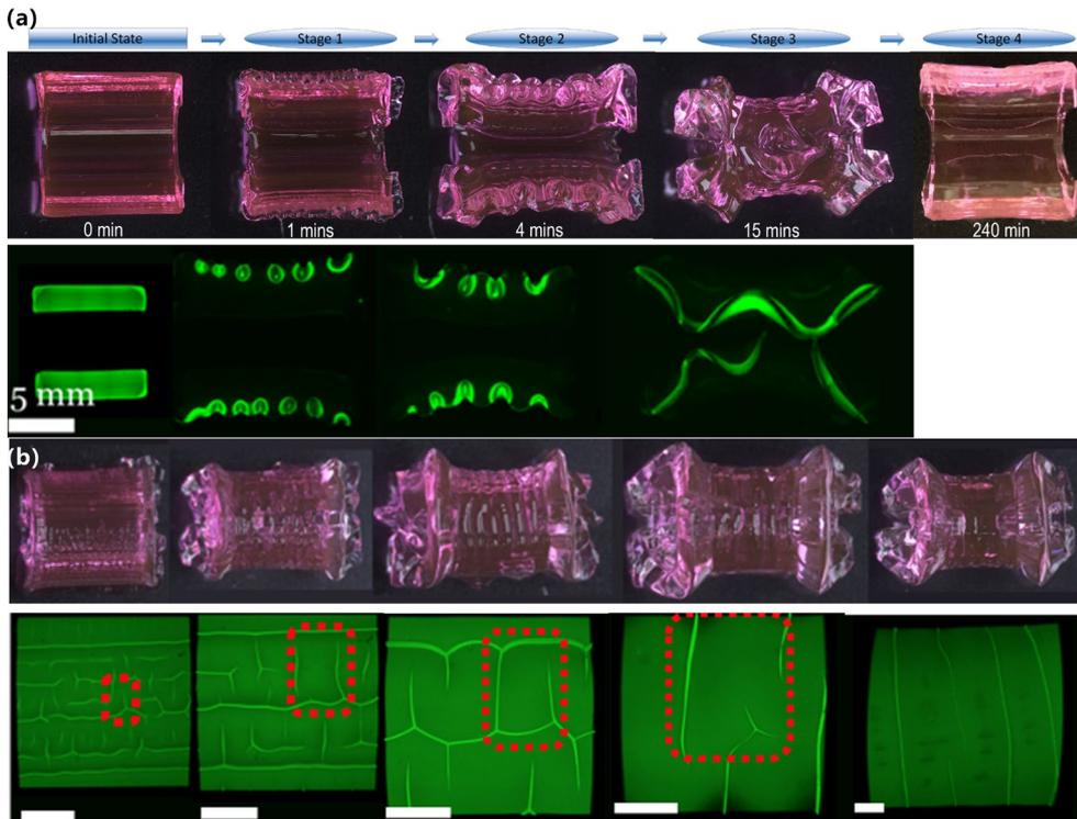
Fig. 1 Morphogenesis of the semi-cylinder at axial direction(a) and circumferential direction(b)
