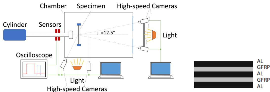
Figure 1. Schematic illustration of the experimental set-up for the gas-gun impact tests.(a) Gas gun (b) Stacking configuration of 3/2 FMLs
