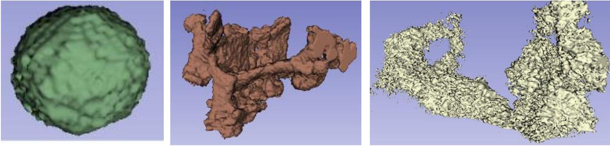
**Figure 3. Microstructural features. Left: Graphite nodule. Middle: Porosity. Right: Carbide structure.**
