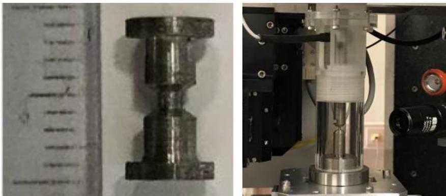
Figure 1. Left: test specimen. Right: test specimen mounted in tensile stage.
