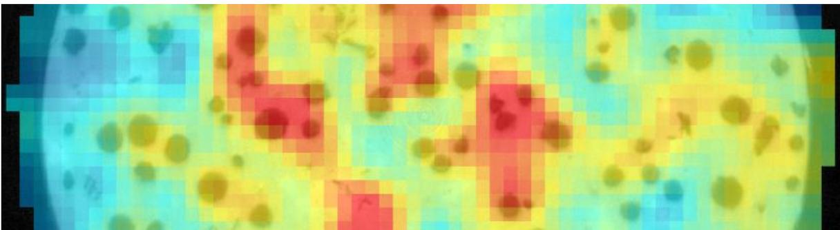
**Figure 4. Maximum normal strain obtained from DVC analysis. Contours range from 0% (blue) to 12% (red). Image corresponds to a load of ~925 N.**
