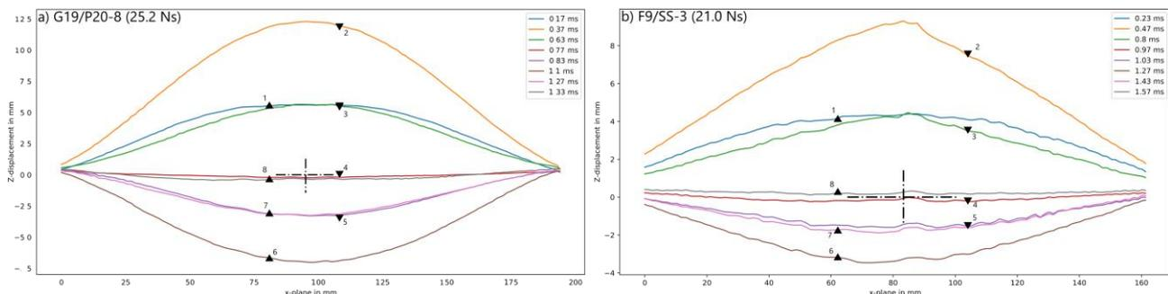
Fig. 3: Deformation profiles of a) (Left hand image) GFRP specimen subjected to 25.2 Ns and b) (Right hand image) flax fibre reinforced Super Sap specimen subjected to 21.0 Ns
