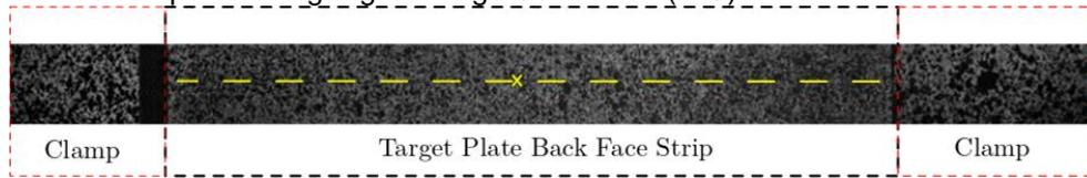
Fig. 2: Example of the speckled central strip captured using high speed cameras
