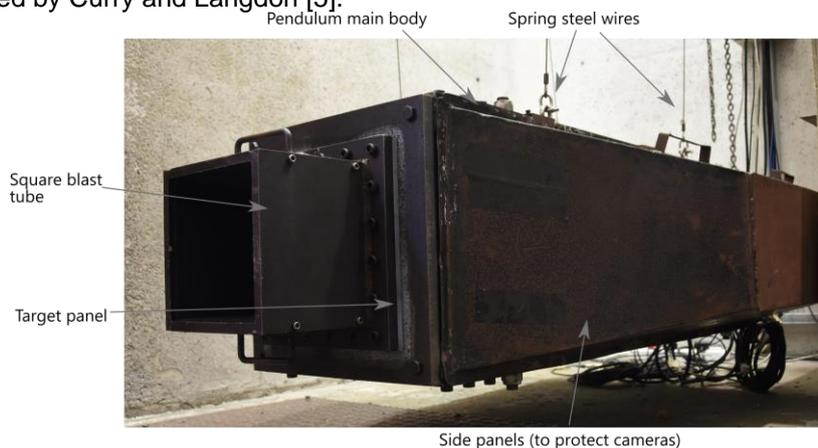
Fig.1: Modified horizontal ballistic pendulum
