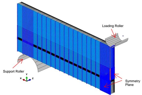
Fig. 2. Finite element model for the SEN(B) specimen with  $B=10\text{mm}$  and  $a/W=0.3$
