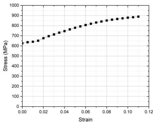
Fig. 1. True stress vs. strain curve of A533B steel under  $-150^{\circ}\text{C}$
