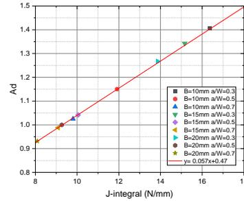
Fig. 3. The correlations between Q,  $\varphi$ ,  $A_p$ ,  $A_d$  and J-integral for different specimens
