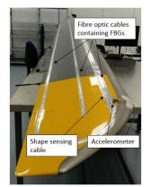
Figure 1: Blade Instrumentation
