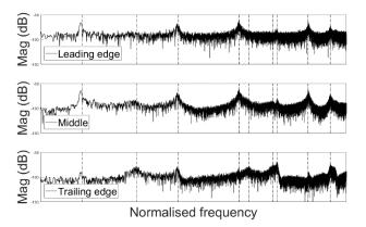
Figure 3: Frequency spectra of three FBGs on the top blade surface in the chord-wise direction at 40% of rotor radius.
