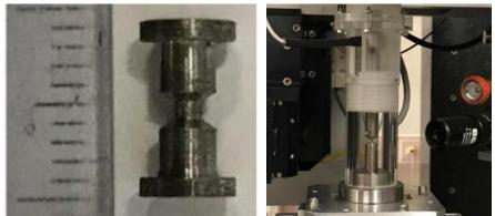
Figure 1. Left: test specimen. Right: test specimen mounted in tensile stage.
