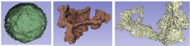
Figure 3. Microstructural features. Left: Graphite nodule. Middle: Porosity. Right: Carbide structure.
