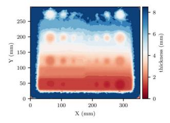
Figure 3: Calculated thickness map
