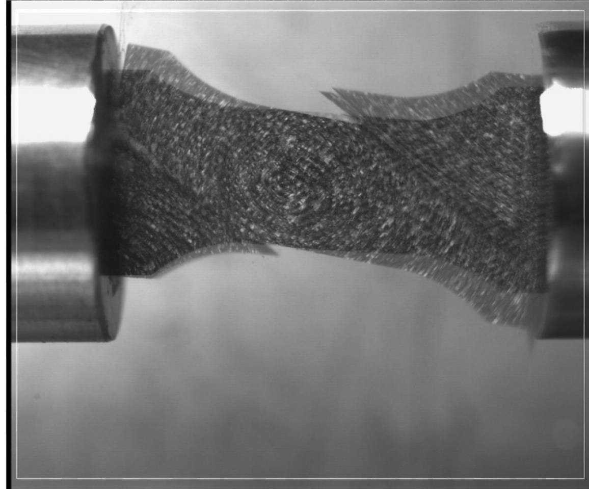
Ghosting if the specimen start deforming
