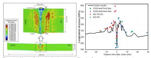
1: Map of measured using the contour method
