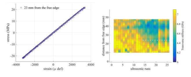
Figure 3: Stress-strain curve just before fracture
