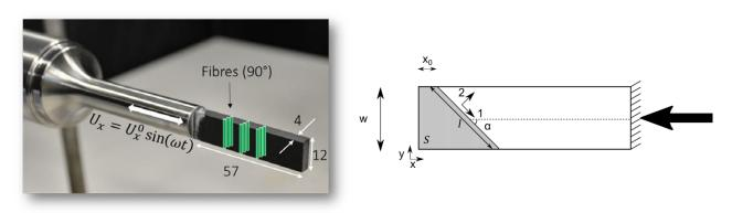
Figure 1: Ultrasonic testing configuration
