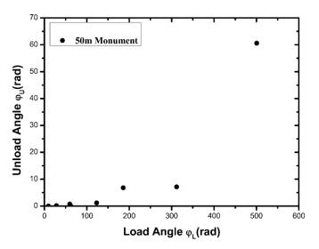
Fig.5: Preliminary data for the 150µm copper wire, gauge length 50m.
