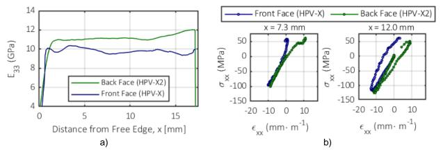
Figure 2: a) Spatial distribution in identified interlaminar stiffness from reconstructed stress-strain curves using the stress-gauge equation (Eq. (1)), and b) sample stress-strain curves reconstructed on from front and back face measurements at two positions on the sample.
