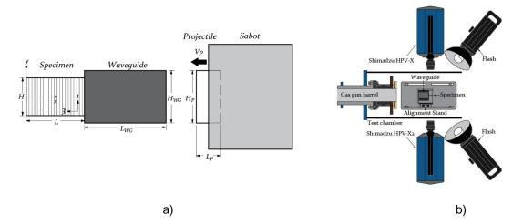
Figure 1: a) Schematic of interlaminar IBII test and b) schematic of the experimental setup with back-to-back cameras used to image the front and back surfaces of the sample.
