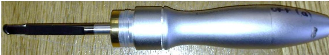
50kHz tuned ultrasonic cutting blade and handpiece
