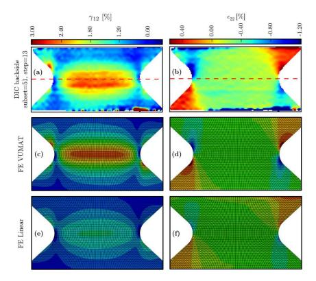
Fig. 2, DIC shear (a) and transverse (b) strain maps; predicted shear (c) and transverse (d) strain maps using the proposed nonlinear user material (VUMAT); predicted shear (e) and transverse (f) strain maps using a linear elastic FE model.
