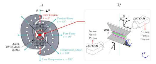
Fig. 1, (a) The Modified Arcan Fixture (MAF) and (b) the butterfly specimen and DIC set-up.
