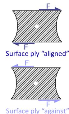
Figure 1b: The two shear orientation cases.
