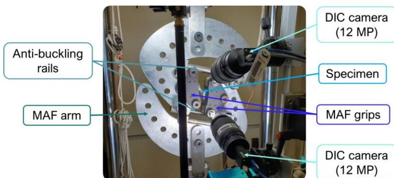
Figure 1a: The experimental setup.
