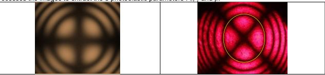
Figure 3 Fringe pattern acquired by diffused light polariscope in conoscopic madality. Unstressed Uniaxial crystal on the left, acquired by diffused light polariscope. Compressed Uniaxial crystal on the right, acquired by laser conoscopic technique; the yellow line is the fitted CL into the first fringe order by which the stress state is evaluated.
