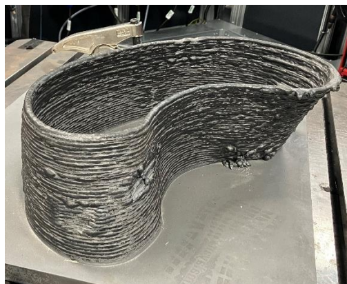
Figure 1. Scaled subsection of the stellarator inner vessel manufactured by WAAM.
