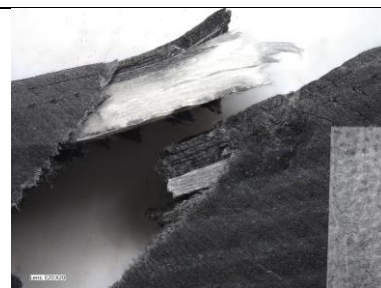
Fig. 2 The sample fractured during the tensile testing.
