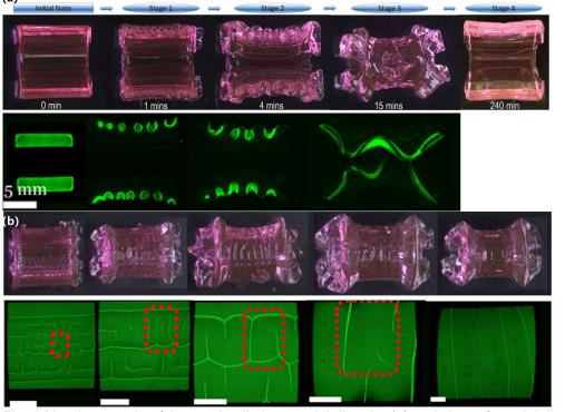
Fig. 1 Morphogenesis of the semi-cylinder at axial direction(a) and circumferential direction(b)
