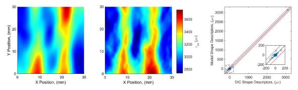
**Fig 2:** Predictions of surface strain (left) and DIC measurements (centre). The validation diagram (right) shows that the model is valid given the uncertainty of the measurement system, the inset shows an enlarged version of the boxed region on the main graph.
