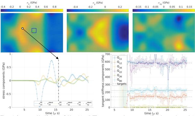
Figure 1: from a to c, identified stress fields at  $16\mu$ s. d) FE vs reconstructed stress at a specific point over time, and e) identified material properties over time
