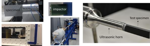
Figure 2: Inertial ultrasonic loading
