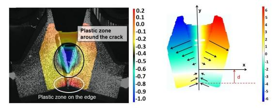
Figure 3: Plots obtained by DIC measurments. Left) Out-of-plane displacement plot in mm, Right) X-displacement plot in mm.
