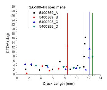
Figure 2: CTOA vs Crack Length plot for two different grades of the same steel.
