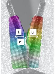
Figure 1: Calculation of CTOA using DIC.
