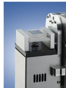
Figure 1 Universal stage with spring sample holder
