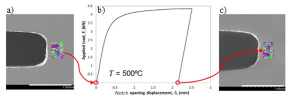
Fig 1: Experimental proceedure: a) Position of the inital EBSD scan, b) Force vs notch opening displacement respons at 500C, c) position of the EBSD scan taken after unloading
