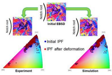
Figure 2: Experimental and simulated change in inverse pole figures (IPF) after deformation at 500C
