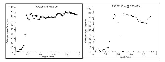
Figure 1 Change in strain angle with applied fatigue loading [1]
