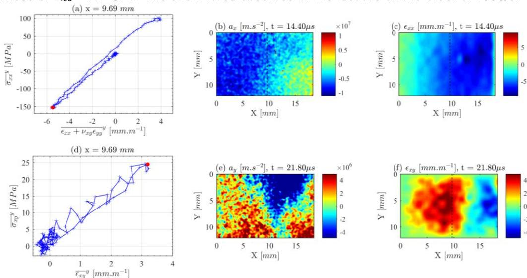
Figure 2: Stress-strain curves and kinematic fields for the axial and shear stress components of an example longitudinal bone sample
