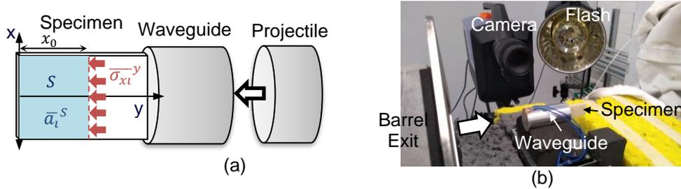
Figure 1: (a) Schematic of the IBII test and (b) photograph of the test set-up
