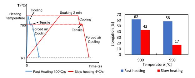
Fig. 1. Non-isothermal tensile tests program (a); effect of heating temperature on elongation (b).
