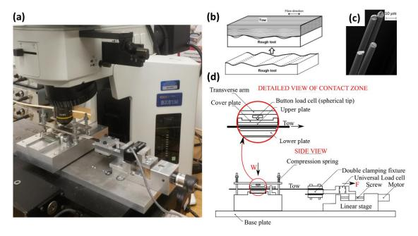
Fig.1: (a) Photo of experimental rig in-situ on microscope stage, (b) schematic of tow-tool contact, (c) SEM micrographs of individual carbon filaments and (d) Schematic side view of experimental rig.
