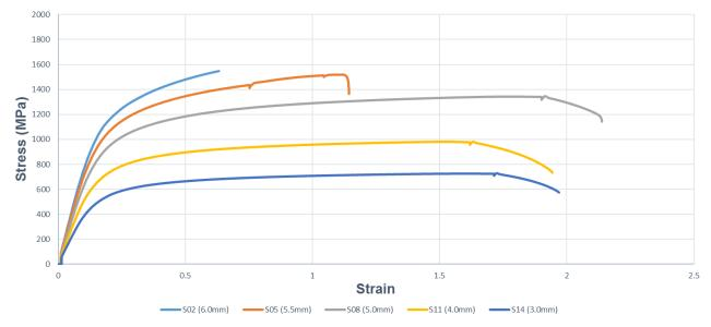
Figure 3: Stress/Strain curves from the ground tensile specimens.
