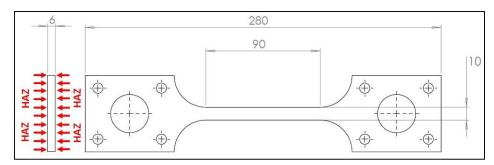
Figure 2: Tensile specimen dimensions (mm)
