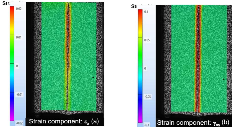
Figure 2 –  $\epsilon_x$  (a) and  $\gamma_{xy}$  (b) distribution just before failure
