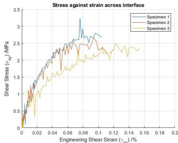
Figure 3 – Shear stress( $\sigma_{xy}$ ) against engineering shear strain( $\gamma_{xy}$ ) for all specimens
