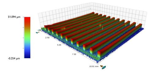
Fig. 1: Optical profilometer scan of structured polycarbonate sample produced by injection moulding, nominal sample area 10x10 mm.
