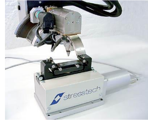
Stresstech 4-point bend system, see www.stresstech.fi for details
