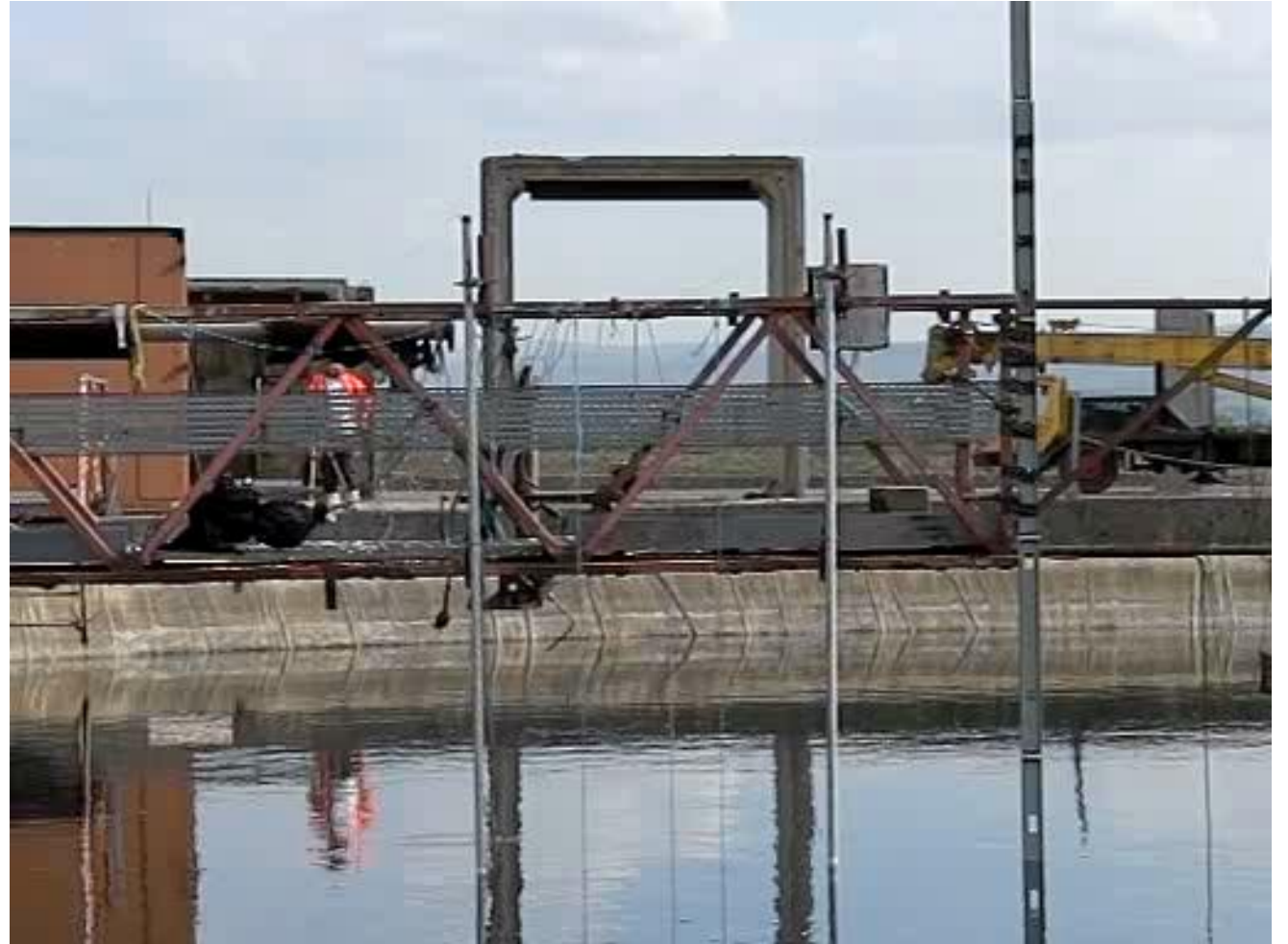
1 kg C4 at 1 m stand-off at 6 m depth Underwater Blast
