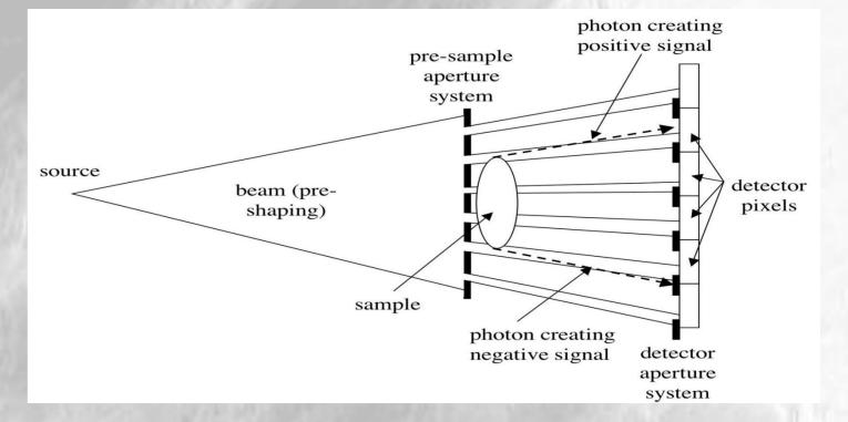
The use of coded apertures makes XPCi feasible in the lab
