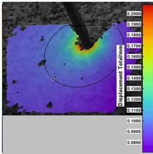
Figure 2 – Displacement across the silicone at 0.5mm penetration
