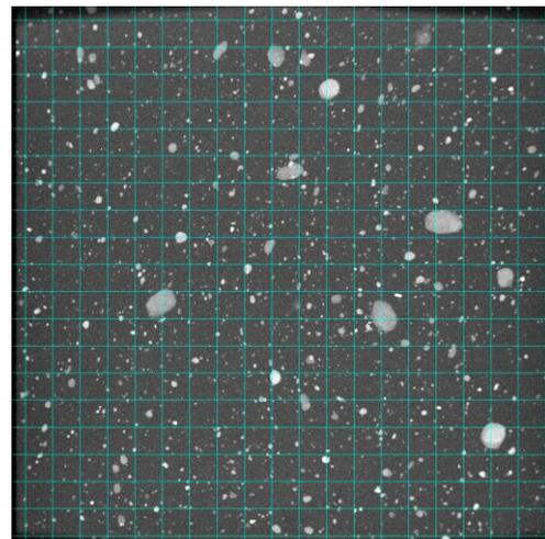
Figure 3 –maximum intensity projection of 100  $\mu$ -CT slices dispersion of titanium dioxide through silicone
